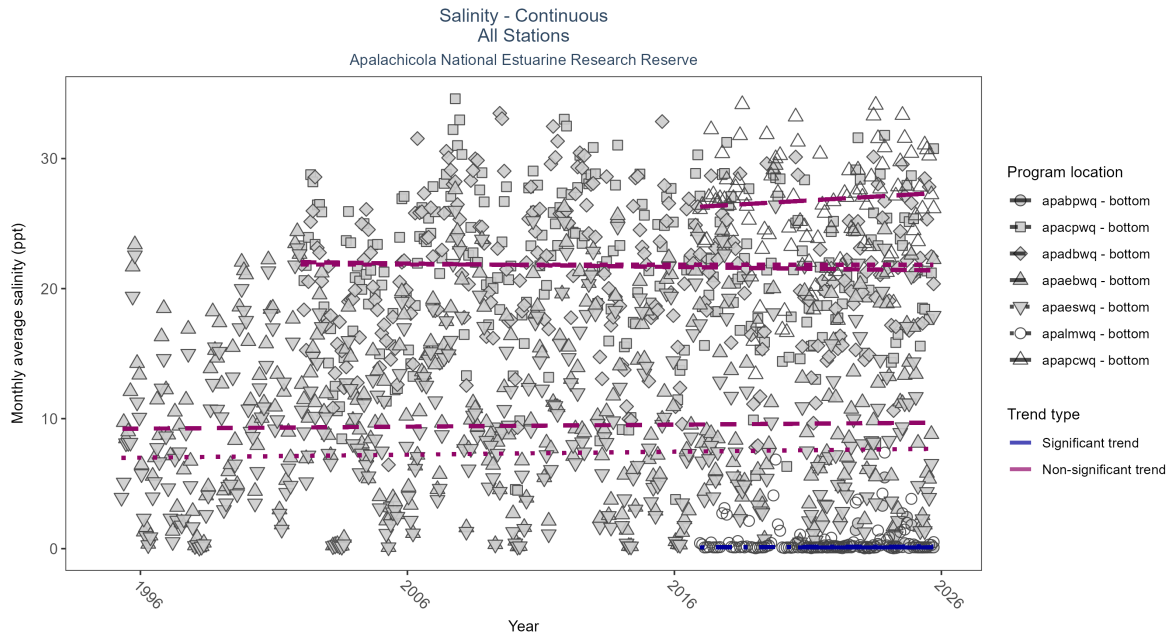
Figure 15: Scatter plot of monthly average salinity over time at continuously monitored program locations. Each location is analyzed separately, with significant (blue) or non-significant (magenta) trend lines shown for time series that included five or more years of observations.
